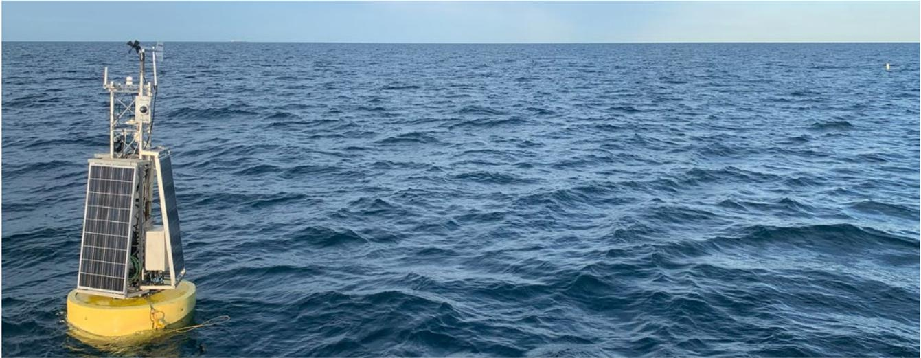
Muskegon Buoy Deployment, July 2020. Taken during the deployment of M20, a NOAA GLERL Real-time Coastal Observation Network (ReCON) buoy, off the coast of Muskegon, MI. NOAA GLERL's ReCON buoys continuously collect meteorological data and provide sub-surface measurements of chemical, biological, and physical parameters. Credit: [NOAA GLERL, 7/30/20](#)
