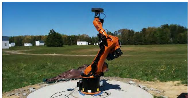
*Top: KUKA 6-axis robotic arm, as installed at NGS’s Testing and Training Facility, with a choking GNSS antenna mounted on the robot’s tool end. Bottom: The robotic arm is housed inside a retractable dome, and is pictured here with several antennas used to validate the system’s results. Image credit: NOAA/NOS/NGS.*
