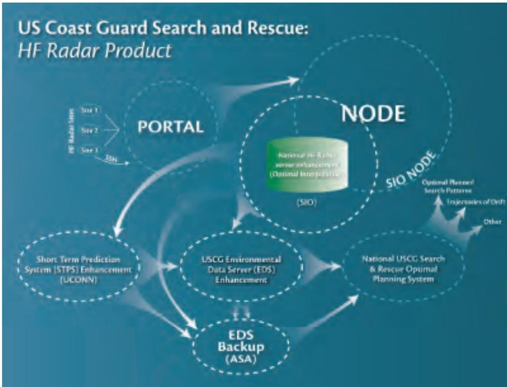
*Schematic of the data pathways and components of the IOOS enhancements to the HF radar component of USCG SAROPS. The blue dotted lines enclose components that existed prior to the project. The enhancements are shown within the white dotted lines.*
